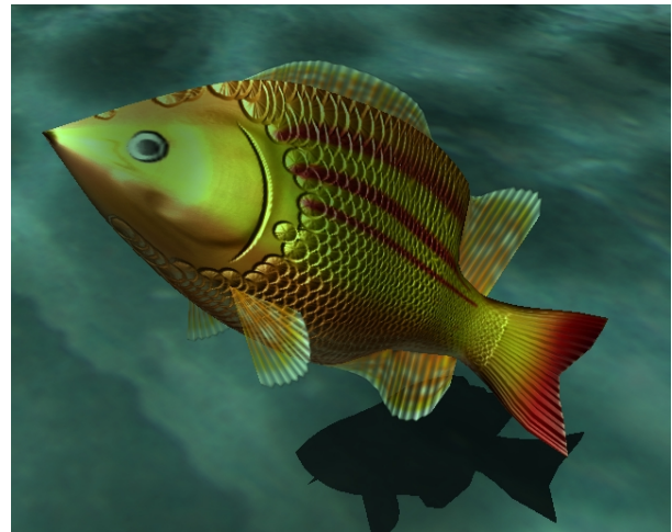
Figure 9: Fish. This scene contains a fish with a bump-mapped body and transparent, bump-mapped fins plus a fragment light that casts a caustic texture on all objects. It runs at 22 frames/sec on a GeForce3.
